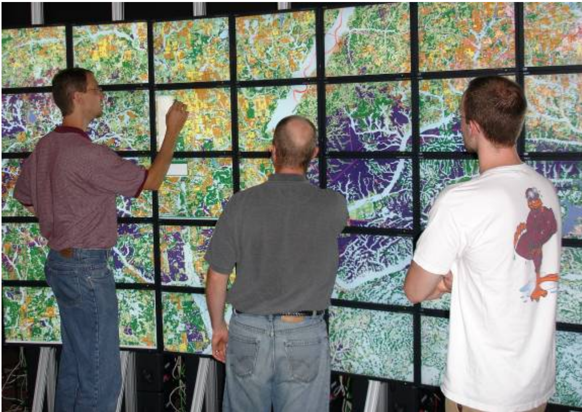
Figure 3. The specific display shown is a 100-million pixel display composed of 50 tiled 20" LCD monitors. The display is approximately 16'x6'. It is controlled by a networked cluster of 25 computers, with software that connects the 50 monitors as though they were a single large high-resolution display surface.
